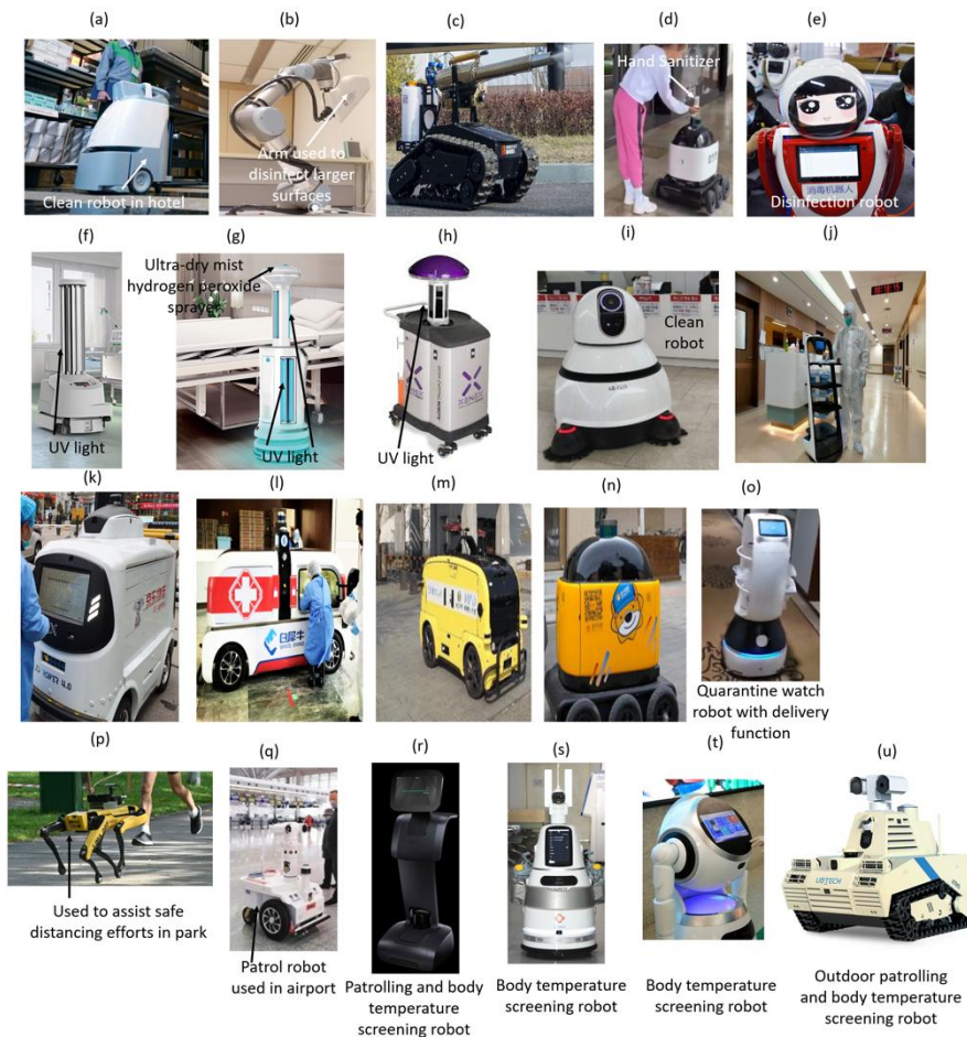
Figure 2. (a) Cleaning Robot from SoftBank Robotics ( courtesy to Ref. [8]). (b) XDBot by Nanyang Technological University ( courtesy to Ref. [9] ). (c) Tank-style, remote-controlled disinfecting robot (courtesy to Ref. [10]). (d) Portable hand sanitizer robot from Zhen Robotics Corp. (courtesy to Ref. [11] ). . (e) Aerosol Disinfection Robot from Shanghai TMiRob Technology (courtesy to Ref. [12]). (f) UV-C light Disinfection Robot by UVD Robots (courtesy to Ref. [13] ). (g) Intelligent Disinfection Robot by TMiRob ( courtesy to Ref. [14] ). (h) UV light robot by Xenex Disinfection Services (courtesy to Ref. [15] ). (i) Autonomous Cleaning Robot by Seoul National University Hospital (courtesy to Ref.[16]). (j) Pudu Technology’s autonomous service delivery robot (courtesy to Ref. [18]). (k) JD Logistics’ large self-driving delivery vehicle (courtesy to Ref. [19]). (l) White Rhino Auto Company’s large self-driving delivery vehicle (courtesy to Ref.[20]). (m) Meituan’s large self-driving delivery vehicle (courtesy to Ref.[21]). (n) ZhenRobotics’ RoboPony (courtesy to Ref. [22]). (o) Quarantine watch robot (courtesy to Ref.[23]). (p) Boston Dynamics’ Spot being used in Bishan-Ang Mo Kio Park, Singapore (courtesy to Ref. [24]). (q) Smart patrol robot being used in Guiyang Airport, China (courtesy to Ref. [25]). (r) Temi robots (courtesy to Ref. [26]). (s) AIMBOT and (t) Cruzr robots from UBTech (courtesy to Ref. [28]). (u) Atris outdoor screening and patrolling robot from UBTech (courtesy to Ref. [30]).
