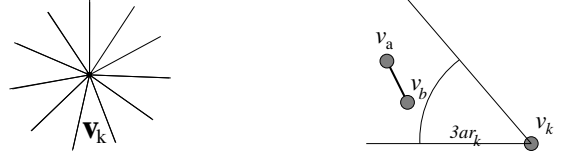
(a) Divide the space into 11 cones (b) Two nodes interfere in same cone
